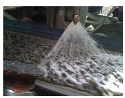
24 L/min = 1,440 L/hr • Dosing rate = 200 parts water to 1 part chemical Chemical usage 0.024L per ton of material
